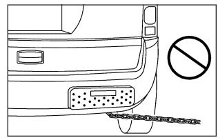
The recovery hook is located at the rear of your vehicle. It can only be used for pulling the vehicle out if it is stuck, not for towing the vehicle.
